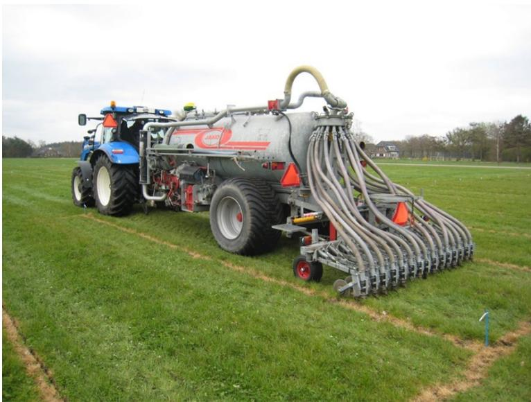
Photo 4. Injector of WUR Unifarm designed for the application of animal slurries. Here adjusted for application of cattle slurry on grassland.
