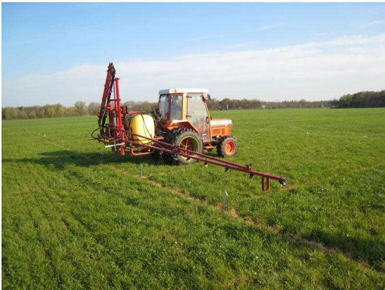
Photo 2. Field sprayer of WUR Unifarm used for application of the liquid mineral nitrogen fertiliser UAN.
