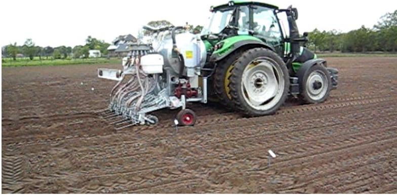
Photo 3. Injector designed for biobased fertilising products. Injector is built by Slootsmid<sup>24</sup> at the request of Inagro<sup>25</sup> and is designed for specific use in field experiments. The design is aimed at mitigating/minimising ammonia losses.
